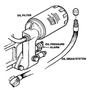
Oil Filter and Oil Drain System
