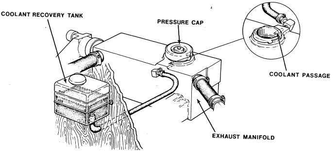
Coolant Recovery Tank, Recommended Installation
