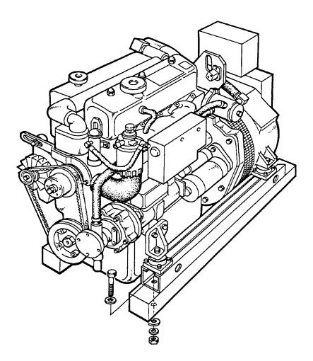
Factors in the location that must be considered are proper support and access for servicing and repairs. There are four 1/2-inch bolt holes in each generator mounting rail to properly secure the generator to its mounting platform.
