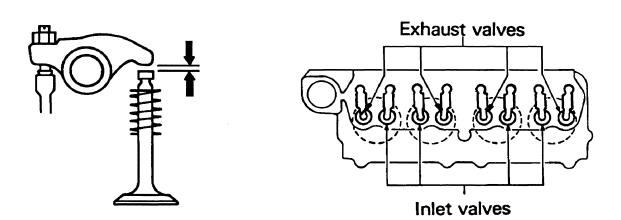
Valve Clearance (engine cold)
