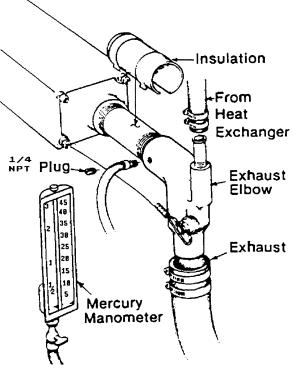
2 inches of mercury 27 inches of water in a water column 15.6 ounces PSI 1.0 PSI
