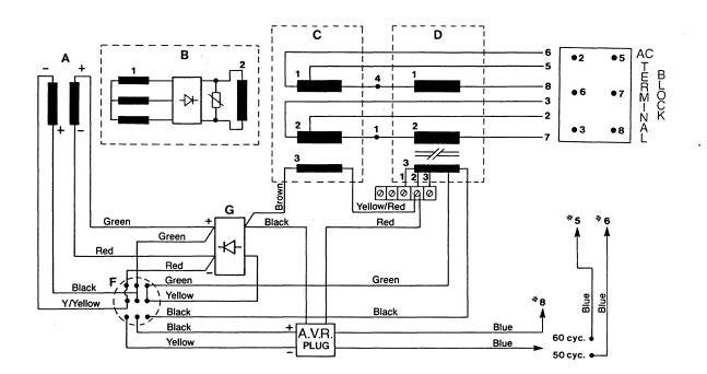
BTD 15.0KW Generator's Internal Wiring Diagram
