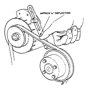
Alternator and Water Pump Belt Tension
