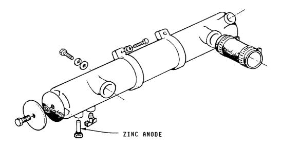
Heat Exchanger Unit of the BTD 15.0KW Generator Set
